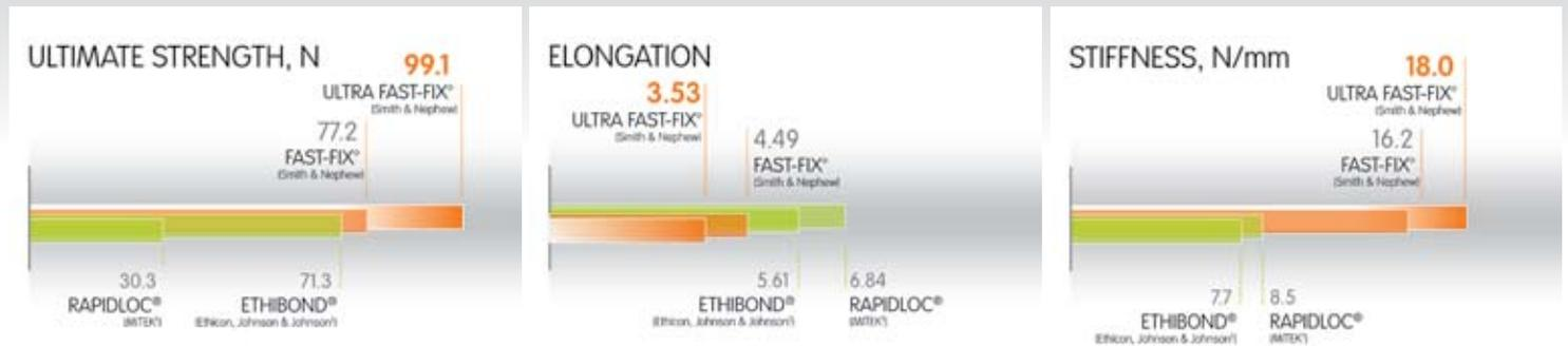
After 1000 cycles between 5N and 20N. All values are means +/- standard errors. Bovine meniscus model.
